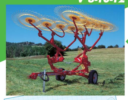
Rake folds into transport position automatically when lifted by means of hydraulic cylinder supplied with the cart.
